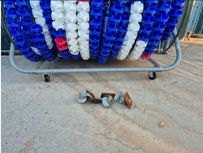
Figure 5. The updated castors for the pool lane rack.
