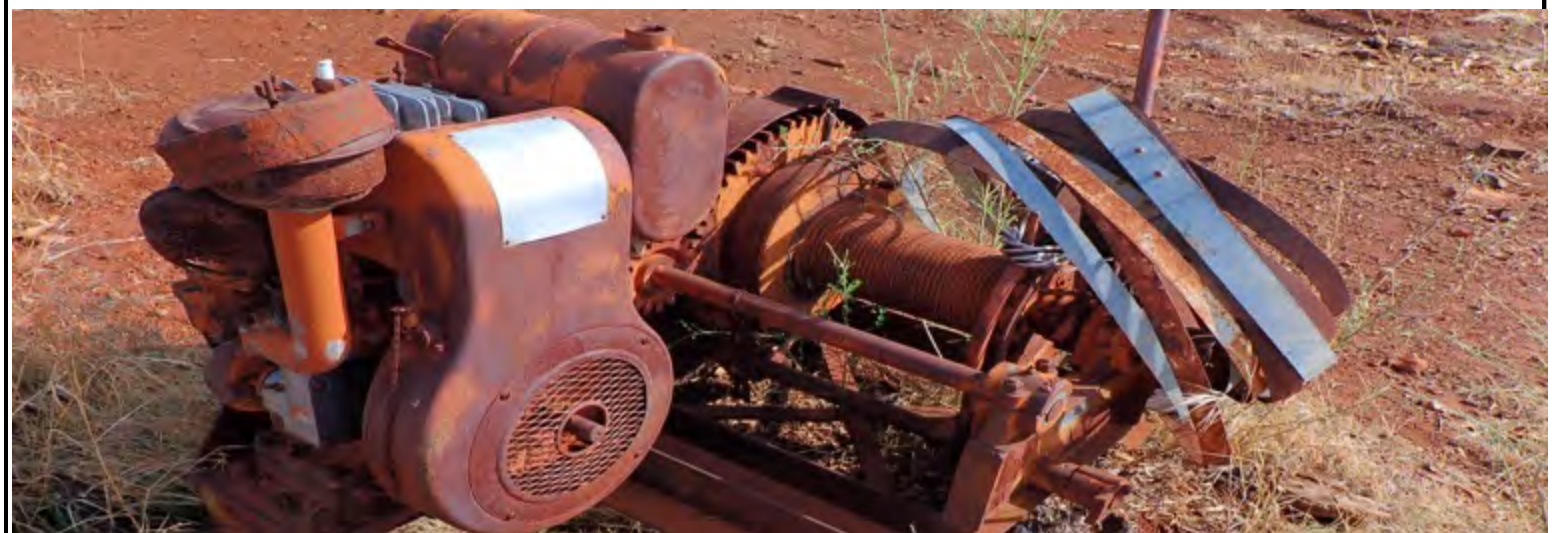
Image 30. Alternative view of rusted Wisconsin Air Cooled Engine.
